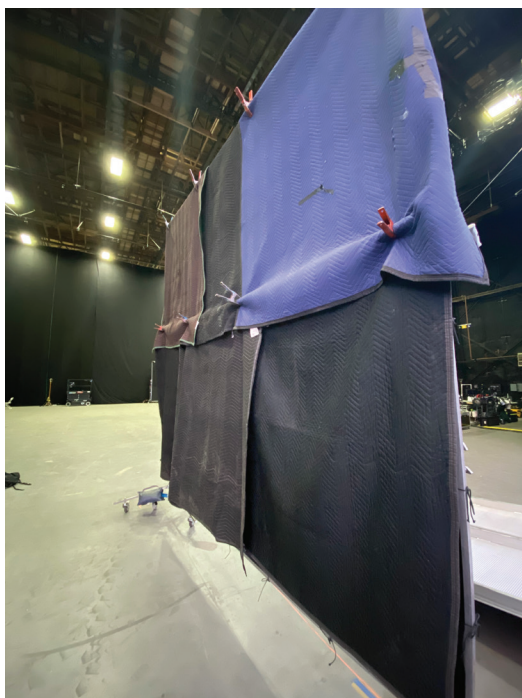
FIGURE 13. Simplest DIY acoustical shade, constructed of furniture blankets, hung over a frame and held up by two (2) C-stands. The one pictured is 12 ft by 12 ft.
