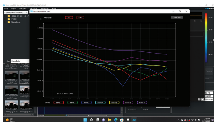
FIGURE 4. Acoustical camera STI calculation (0.51) of balloon pop sonic instance recorded in an empty LED volumetric stage without acoustical mitigation elements. Bands 1-7 depict standard STI frequencies of 125, 250, 500, 1K, 2K, 4K, 8K, respectively.
