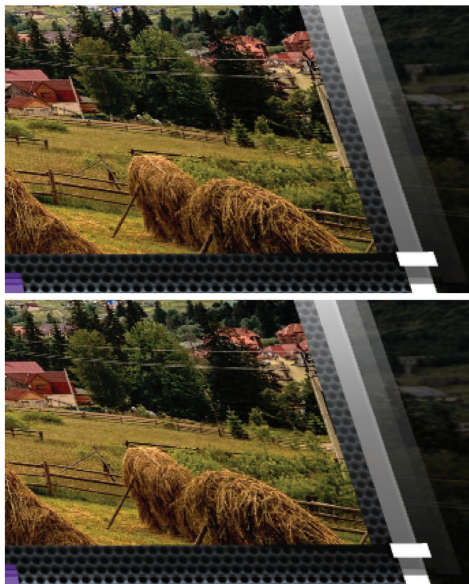
FIGURE 9. Comparison (500% zoom) of uncompressed original (top) and 444 SQ compressed (bottom).
