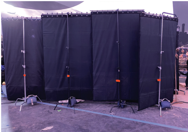
FIGURE 15. Zero-reflection (ZR) screens from Delta H. Designs, Inc. configured in a large LED volume stage, along with standard floor mats and furniture blankets.
