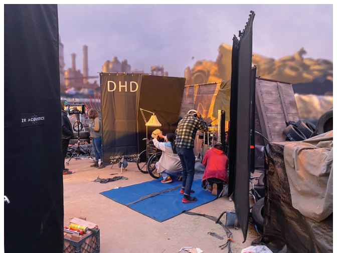
FIGURE 17. Zero-reflection (ZR) screens placed in an active set behind camera to capture sound originating from the actors and shield the actors from sound reflecting at them from the walls and outside the stage opening.
