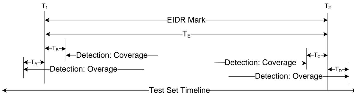
**Figure 6 –Metrics based on Accuracy of Detection**
