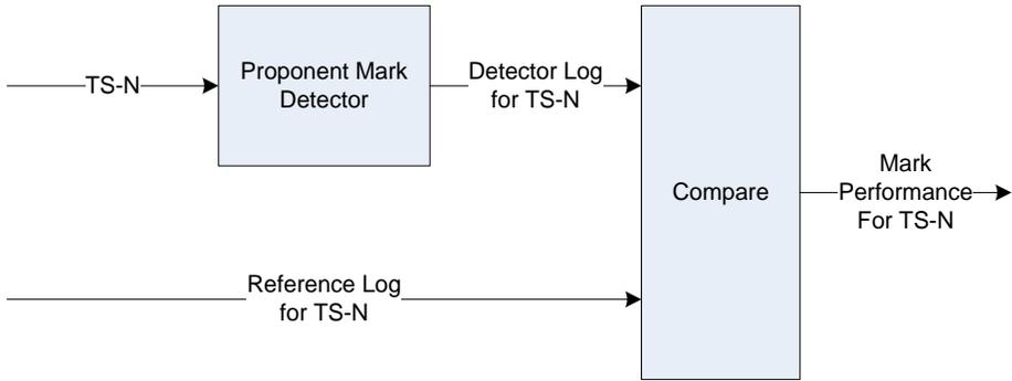
**Figure 3 – Block Diagram of Detection and Performance Measurement Process**
